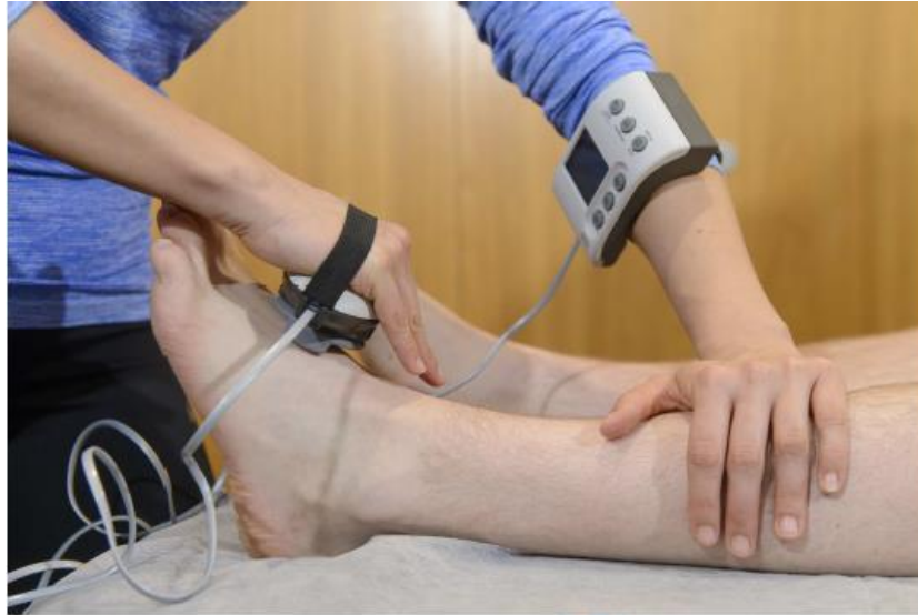
Figure 16. A hand-held dynamometer is used to assess ankle joint isometric dorsiflexion strength.
